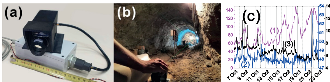
Fig.1. (a) Microlidar, (b) BNO hot tunnel, (c) gas emanation in the hot tunnel: radon (1), \text{H}_2\text{O} (2) and aerosol (3).
