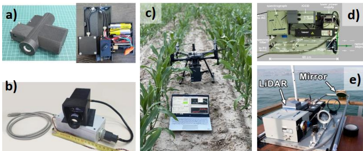
Fig. 1. Compact fluorescence (a) and eye-safe (b) LIDAR systems developed at Prokhorov General Physics Institute of RAS. Compact LIDAR installed at a small drone (c). Raman LIDAR (d) developed for fresh and seawater monitoring (e).
